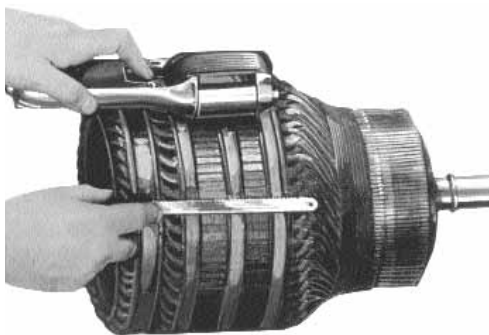
Type U-2 Universal Adjustable Growler may be used as both an external Growler for armatures and an Internal Growler for stators.
